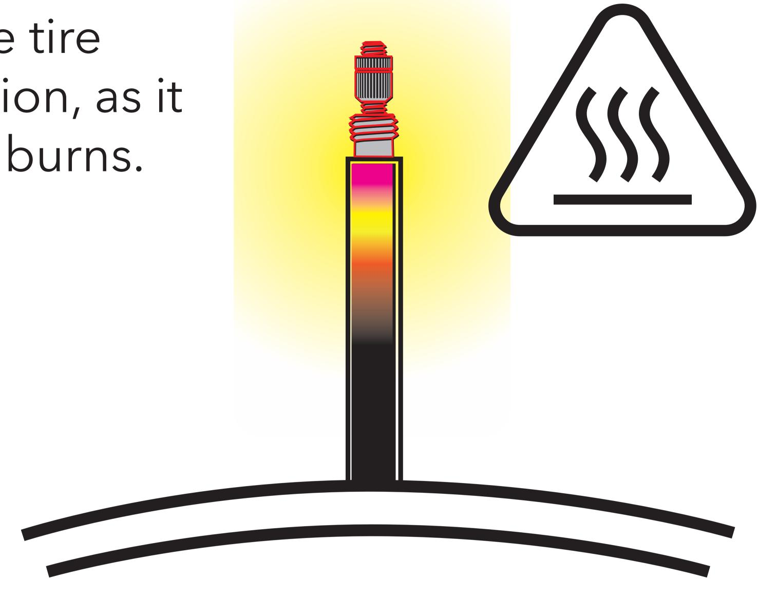
**CAUTION** - For **TPU** inner **tubes with resin valves**, use the extension hose to prevent overheating damage to the valve.
