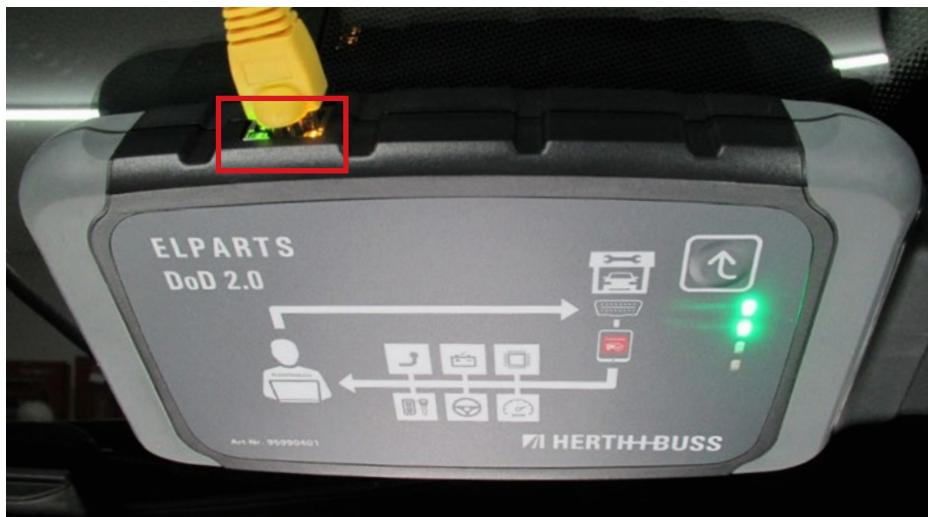
Both LEDs are permanently lit. The VCI is connected to the server and you can use the DoD service. A reset of the VCI is necessary if it is to be integrated into another Wifi network. The VCI must be supplied with voltage via an OBD socket.
