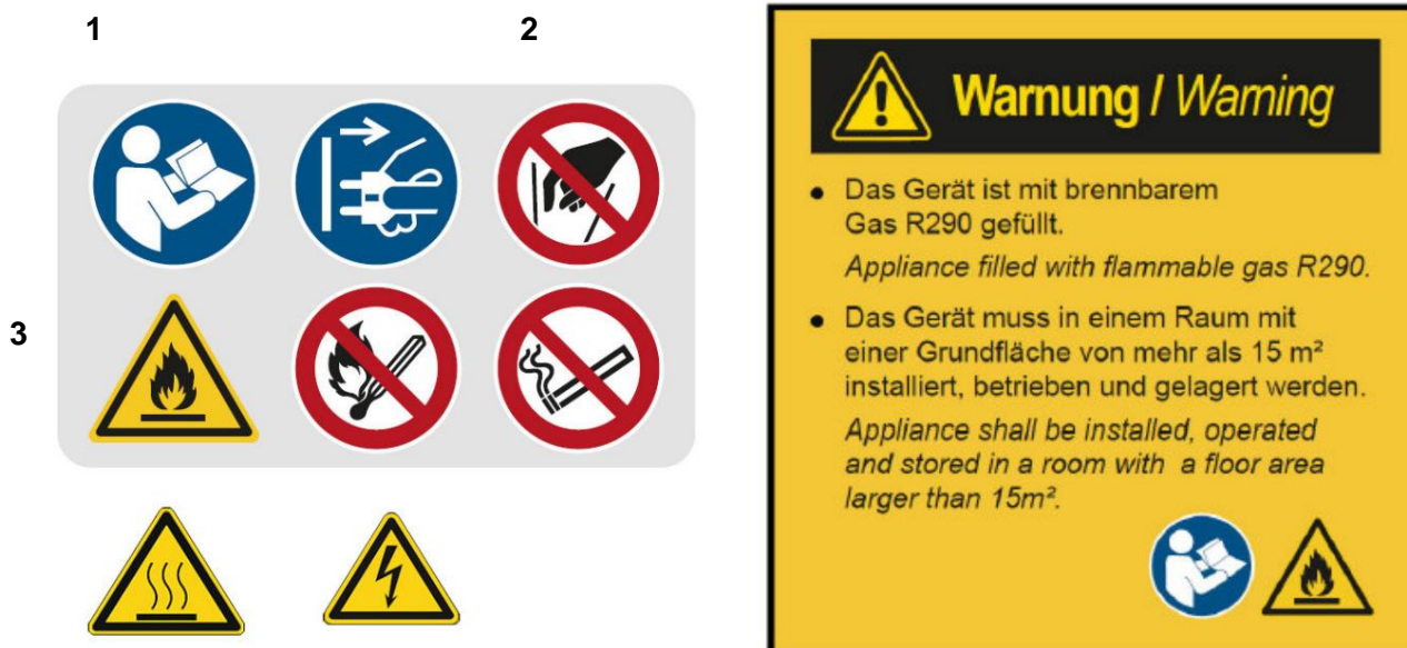
Fig. 1-1: Safety markings: 1 Mandatory sign: Observe operating instructions, unplug the power cord | 2 Prohibition sign: No reaching inside, no open flame; fire, smoking prohibited | 3 Warning sign: Warning of flammable substances, warning of hot surface, warning of electrical voltage
