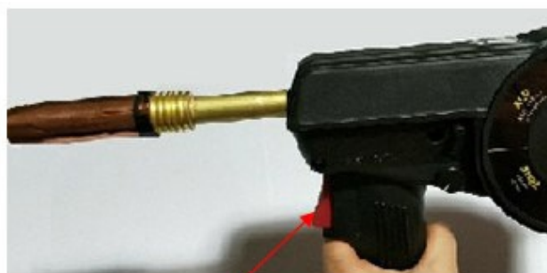
11. Pull the trigger to push the wire down the neck until it emerges from the contact tip.
