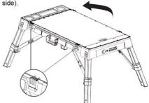
3. Remove the panel, turn it over so that the anti-slip work platform surface is face up, and place it back onto the platform, Re-fasten all four latches.
