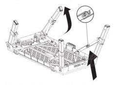
3. Press the spring button on each leg and pull each leg out until the spring button clicks again.
