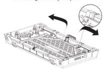
2. Pull each leg up and out and extend hinged bracket until it locks in place.
