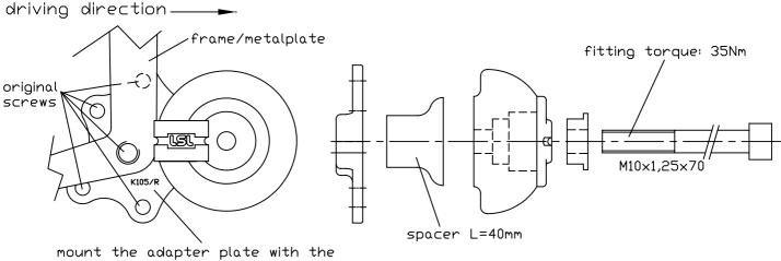
mount the adapter plate with the identification K105/R instead of the original metalbracket between the cylinder head and the frame/metalplate. Use the original screws.
