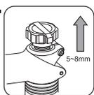
Counterclock-wise loosen the cap by hand or use the lever if it's too tight.
