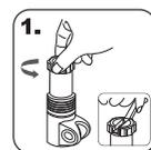
Loosen to remove the cap. Use lever if the nut cap is too tight.
