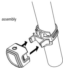
Slide the rear light onto the mounting clip until the rear light clicks into place.
