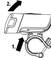
1. Press release button on underside and remove front headlamp (2.)
