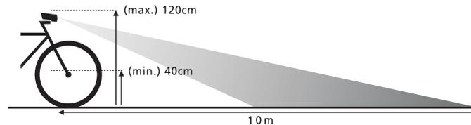
Align the LED front light so that the light beam reaches the road approx. 10 meters in front of the wheel (see ill.). The light beam of the LED front light must point straight in direction from 400 up to 1200mm.
