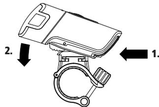
1. Put on the front headlight on rear edge of bracket
