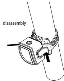
Activate the release lever on both sides (simultaneously) and remove the rear light.
