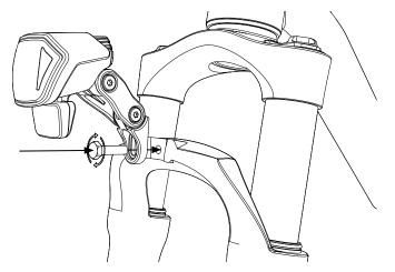
Front light (1) mount to the steel bracket and make sure that the front light (1) cannot be adjust by itself (tighten the screw firmly enough!)
