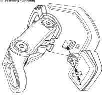
It is possible to mount a white reflector (2) to the bottom of the front light (1). The reflector is equipped with two pins that adapt into the holes of the front light. Screw the reflector to the front light for a permanent attachment.
