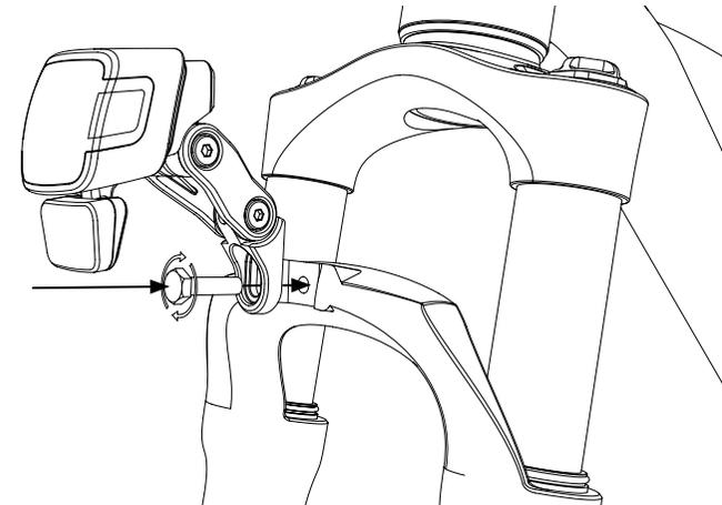
Front light ① mount to the steel bracket and make sure that the front light ① cannot be adjust by itself (tighten the screw firmly enough!)
