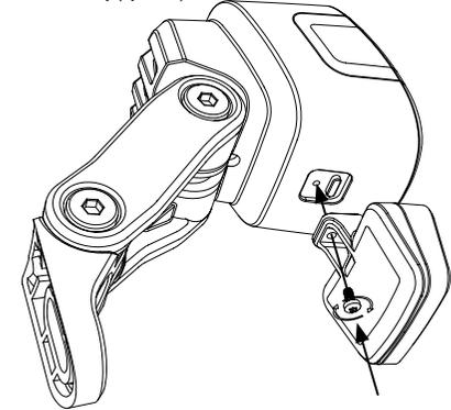
It is possible to mount a white reflector ② to the bottom of the front light ①. The reflector is equipped with two pins that adapt into the holes of the front light. Screw the reflector to the front light for a permanent attachment.
